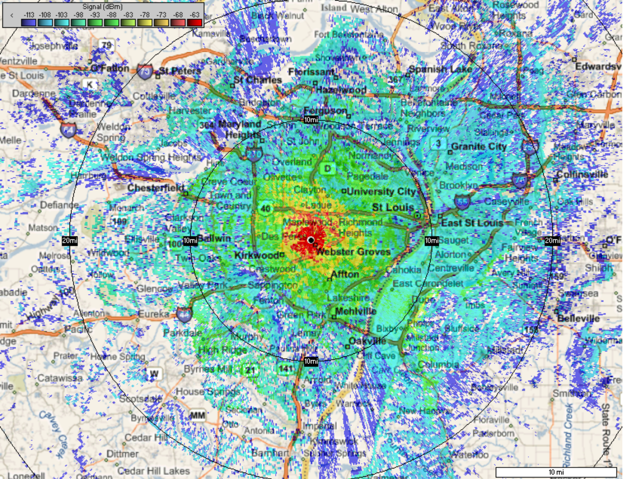
Sample Site (200' Tower - 50 Watt Digital Repeater) Talk-Out to Portable (shown w/ optional distance rings)
